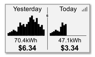
The graphs show hourly data, with a bar for each hour. The height of the bars is proportional to the number of kWh consumed for each hour. The graphs are autoscaling, and meant to show relative, rather than absolute values. The small number
