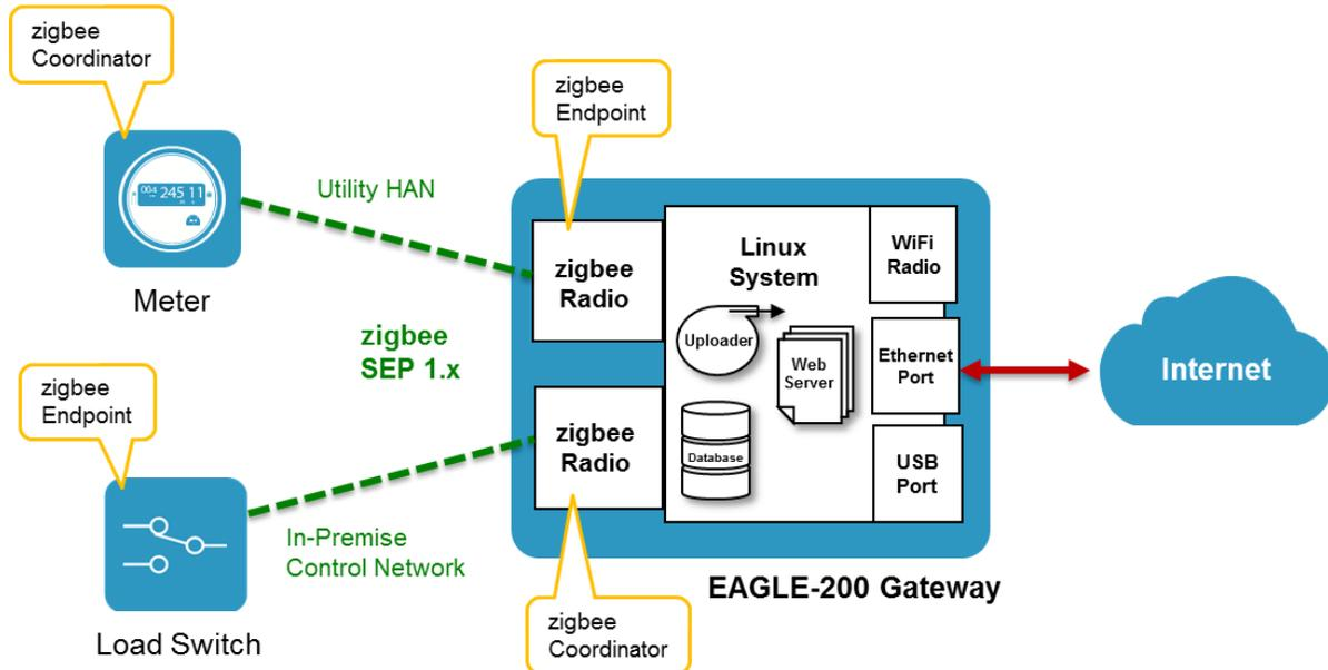
Utility HAN: The first zigbee radio in the EAGLE communicates directly with a smart meter equipped with zigbee wireless capability that supports the Smart Energy Profile (SEP) protocol standard (almost all US smart meters support this standard). This is called the Home Area Network (HAN). It consists of the utility smart meter, which is the network Coordinator, and one or more Endpoints. The EAGLE acts as an Endpoint on the HAN. The EAGLE sees the utility meter as an “electric\_meter” device.
